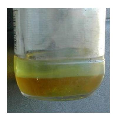
When ethanol blended gasoline reaches its saturation point because of contamination with H<sub>2</sub>O, multiple layers are formed. The top layer is gasoline with a lower octane rating, and the bottom is a mixture of water and ethanol that will not ignite during engine combustion. If ethanol blended gasoline reaches this state, a phenomenon known as "Phase Separation," the engine can be detrimentally affected.
